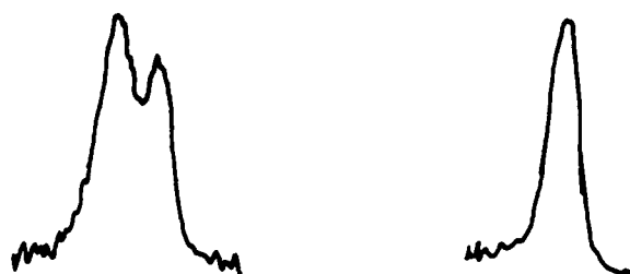
Fig. 3.—Double resonance experiment on IV. Before irradiation of the bridgehead proton the cyclobutene proton appears as a doublet ( J = 0.86 c.p.s.). After irradiation of the bridgehead proton the doublet collapses to a singlet.
